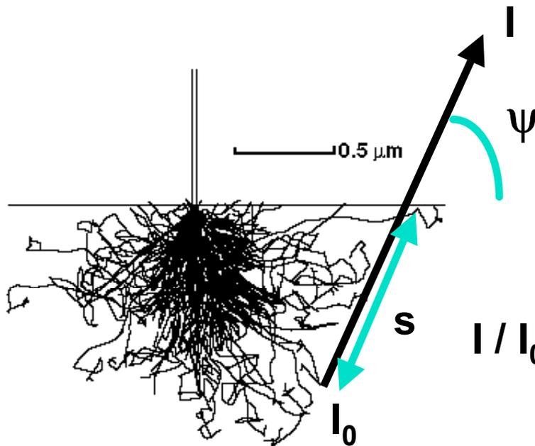
A: X-ray absorption within the specimen reduces the intensity emitted.
